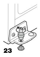
**23.** Fit adjustable foot from underneath and attach hinge pin to it.
