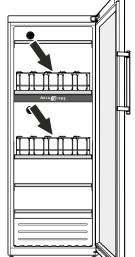
Slide the support bars ① into the required position.
