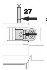
**27.** Push in hinge pin until groove in the pin lines up with bore hole in the hinge bracket.
