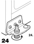
**24.** Insert pin fully into hinge bracket and tighten adjustable foot by hand.
