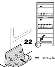
22. Screw hinge bracket into place.
