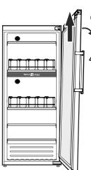
4. Tilt door slightly to the side and remove by lifting upwards.
