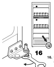
**16.** Undo adjustable foot with the spanner provided.
