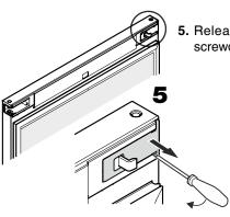
5. Release cover with a small screwdriver and remove.
