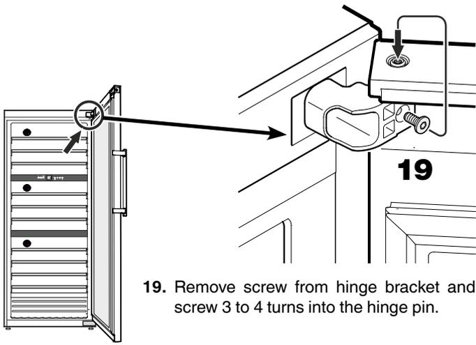
**19.** Remove screw from hinge bracket and screw 3 to 4 turns into the hinge pin.
