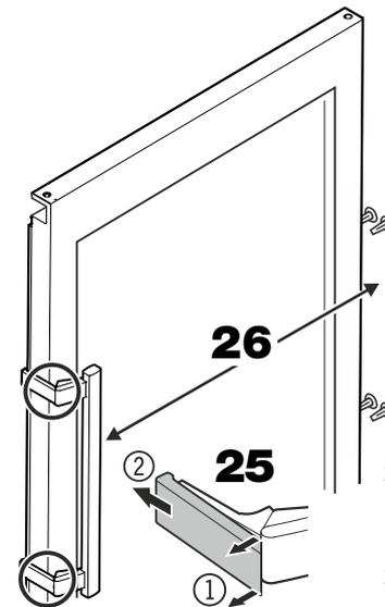
**25.** Release pressure plates at the front ① and pull them backwards to remove ②.
