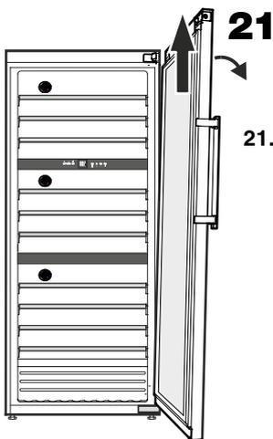
**21.** Tilt door slightly to the side and remove by lifting upwards.
