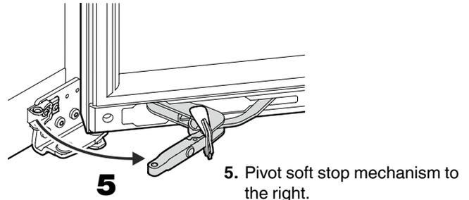
5. Pivot soft stop mechanism to the right.
