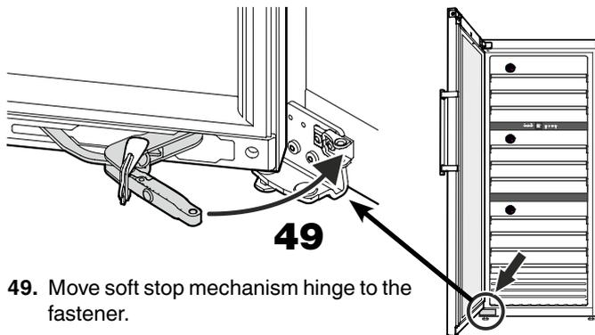
**49.** Move soft stop mechanism hinge to the fastener.
