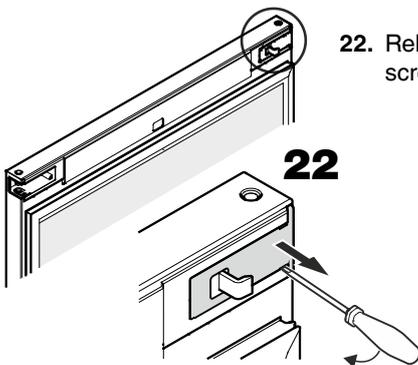
**22.** Release cover with a small screwdriver and remove.
