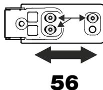
**56.** Undo screws and slide hinge bracket to the right or left.
