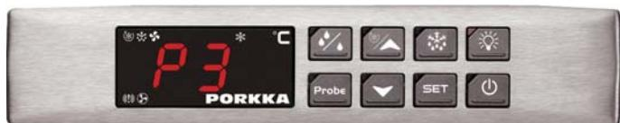
**"P3"**      Condenser probe failure\*\*\*
