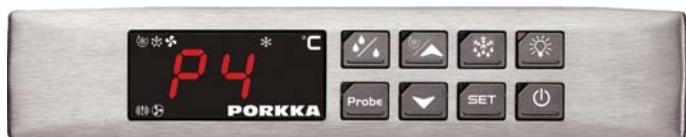
**"P4"**      Extra probe failure\*\*\*
