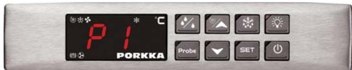
**"P1"**      Thermostat probe failure\*\*\*
