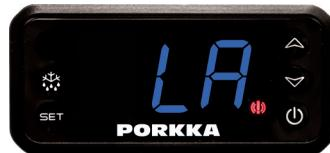
Reset the alarm signal by pushing **SET** key.
